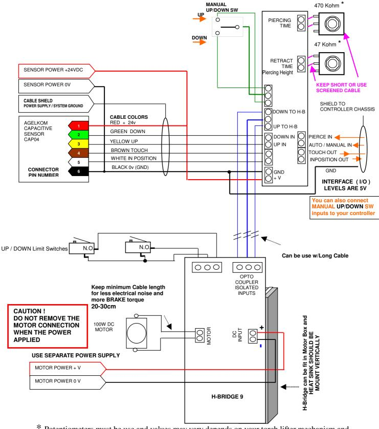
\* Potentiometers <u>must be use</u> and values may vary depends on your torch lifter mechanism and piercing time request of plasma generator.
